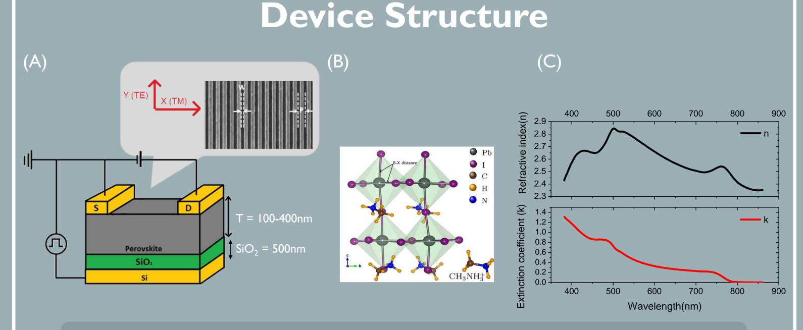
A:Transistor Schematic inset: Optical microscope image of nanograting B: MAPbl<sub>3</sub> crystal structure [4] C: Optical constants of MAPbl<sub>3</sub> at 300 K
